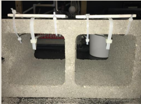
Side view of settlement sampler with settlement plates
