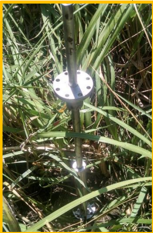
2017 - Due to very high sediment deposition, rod extended and collar raised
